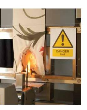
You can use FlexiBurn for testing the ignition and flame spread properties of apparel, curtains, drapes, nightwear, toys, protective clothing, technical fabrics, building and other materials.
