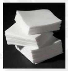
The crocking test is based on assessing the amount of dye transferred from the specimen under test to a standardised crocking cloth.
