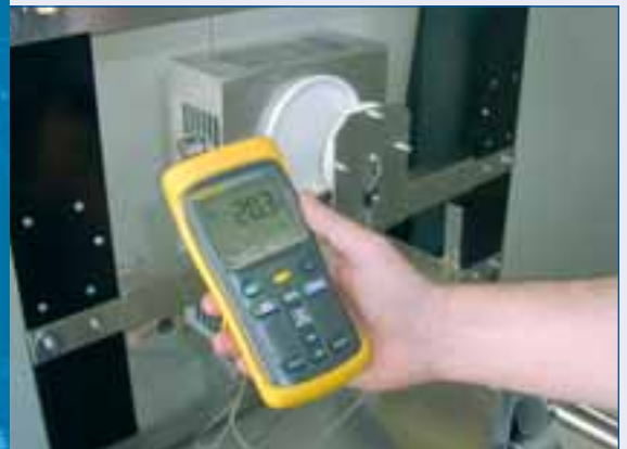
CALIBRATION OF RADIATOR WITH COPPER DISC CALORIMETER
